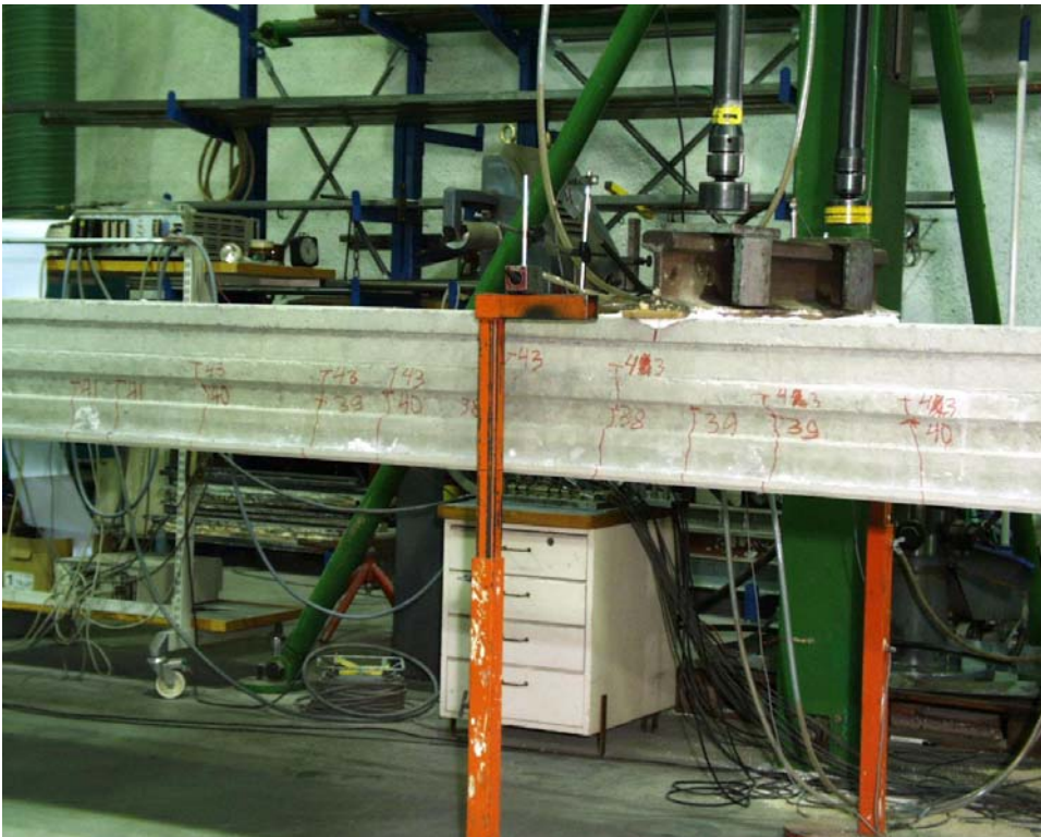
Fig. 6. Location of flexural cracks in eastern slab.
