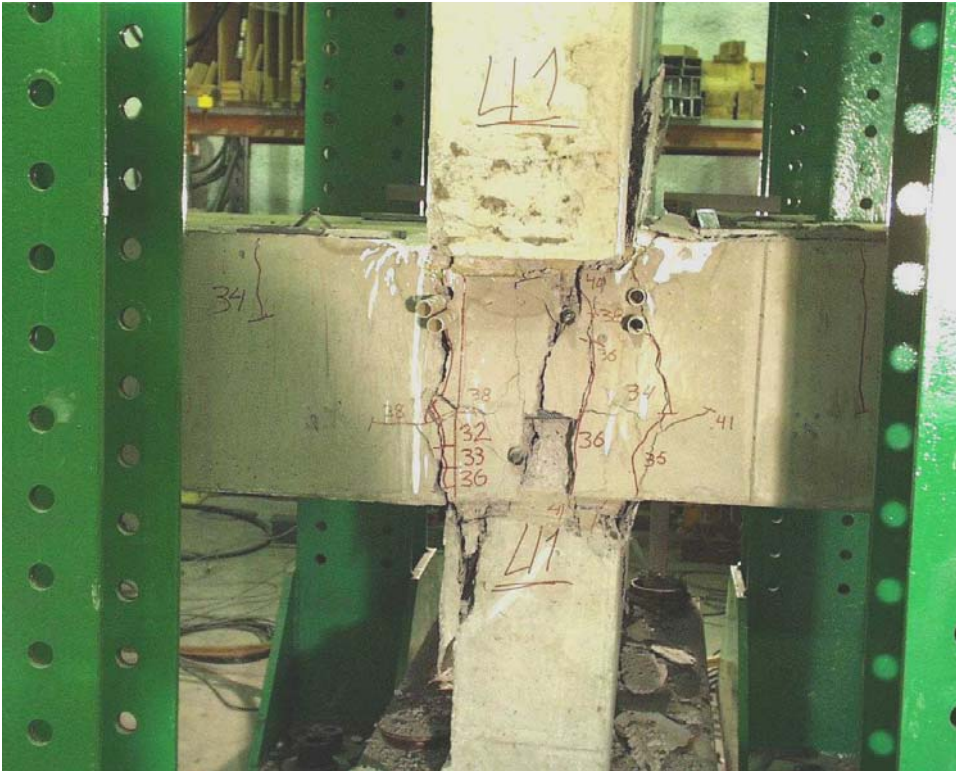
Fig. 9. Cracking pattern after failure seen from north.
