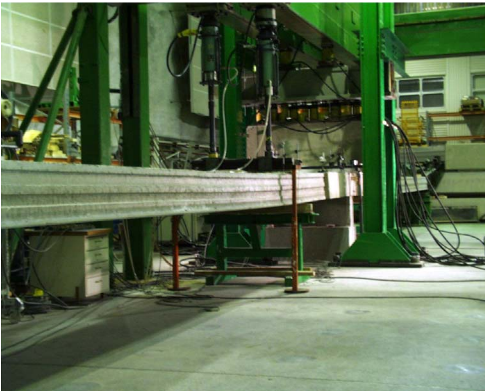
Fig. 8. Deformation of the eastern slab before failure.
