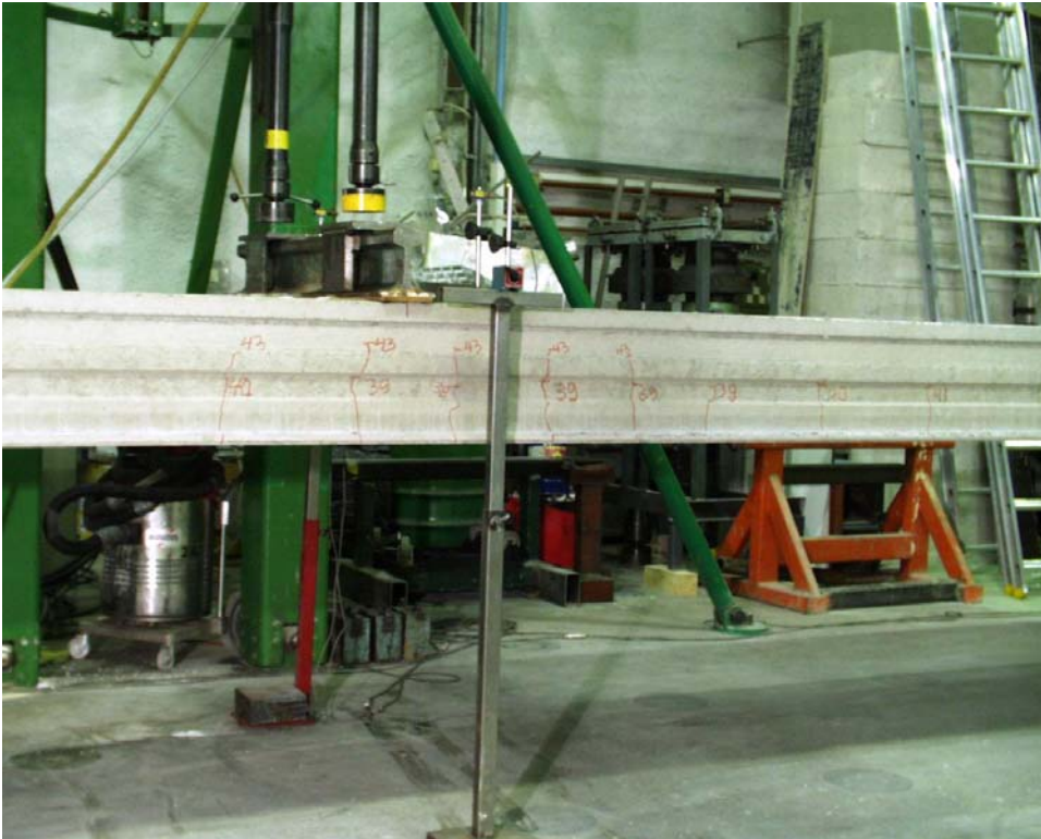
Fig. 5. Location of flexural cracks in western slab.
