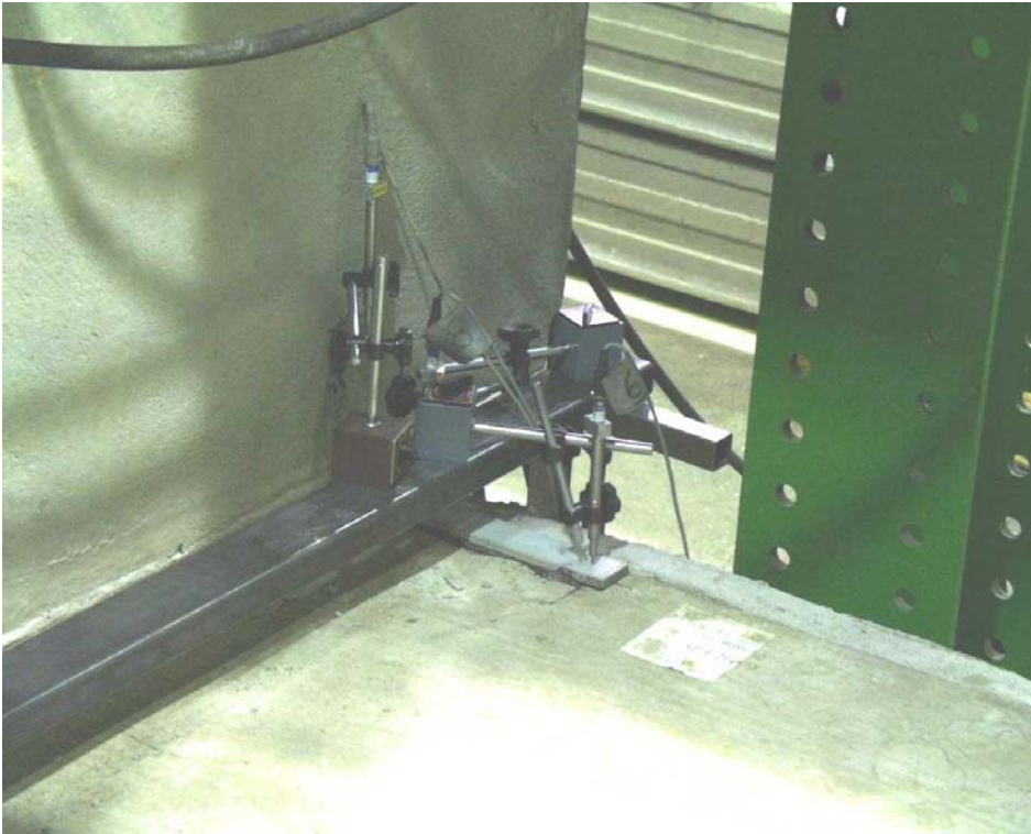
Fig. 5. Inductive transducers for measuring vertical displacements.
