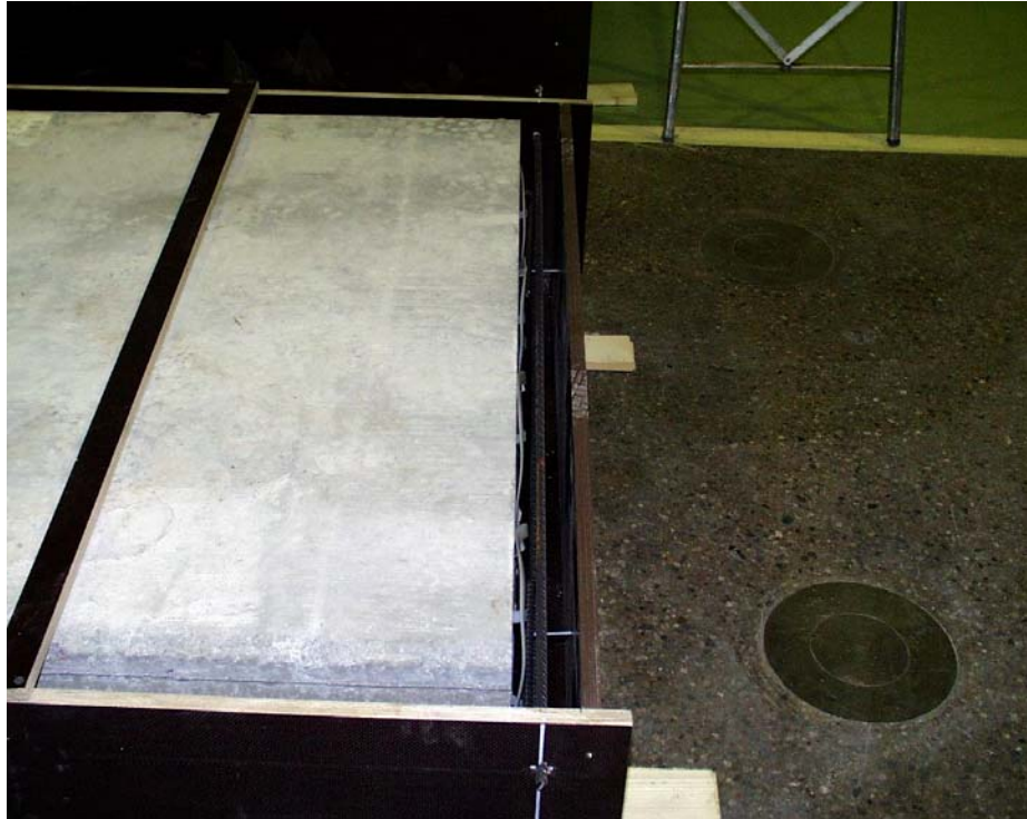
Fig. 3. End of test specimen before grouting.
