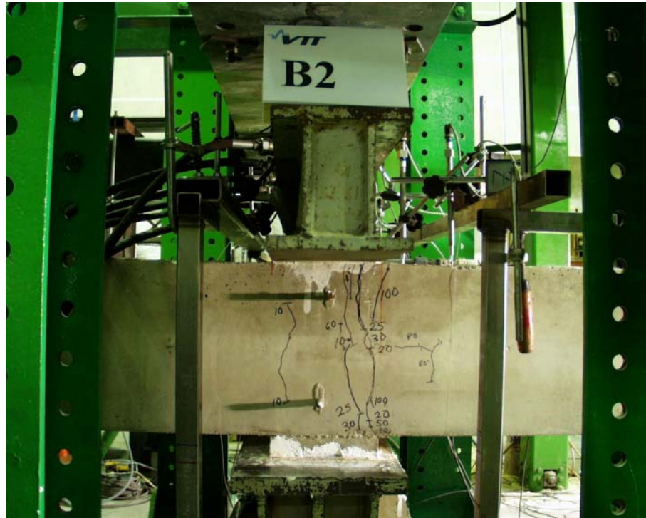
Fig. 25. B2, North edge. First cracks.
