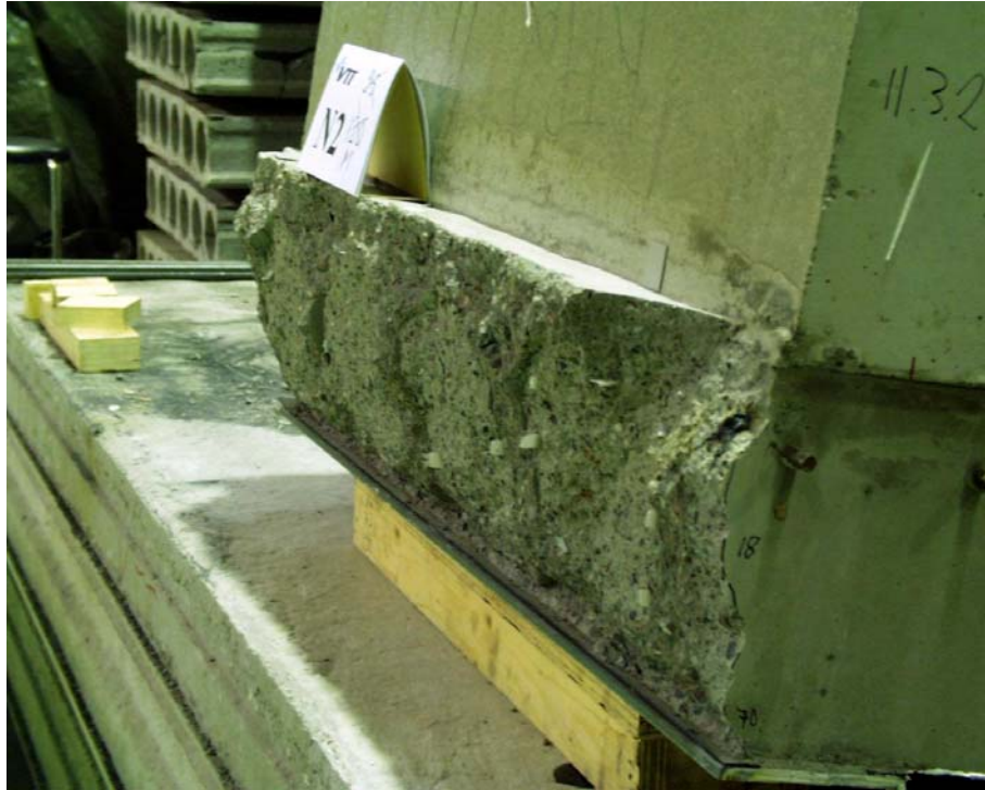
Fig. 35. N2. Flexural crack.
