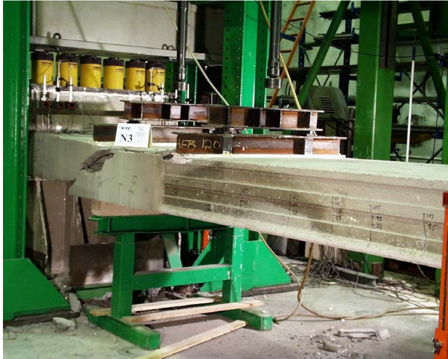
Fig. 41. N3, North edge. Failure crack and flexural cracks.
