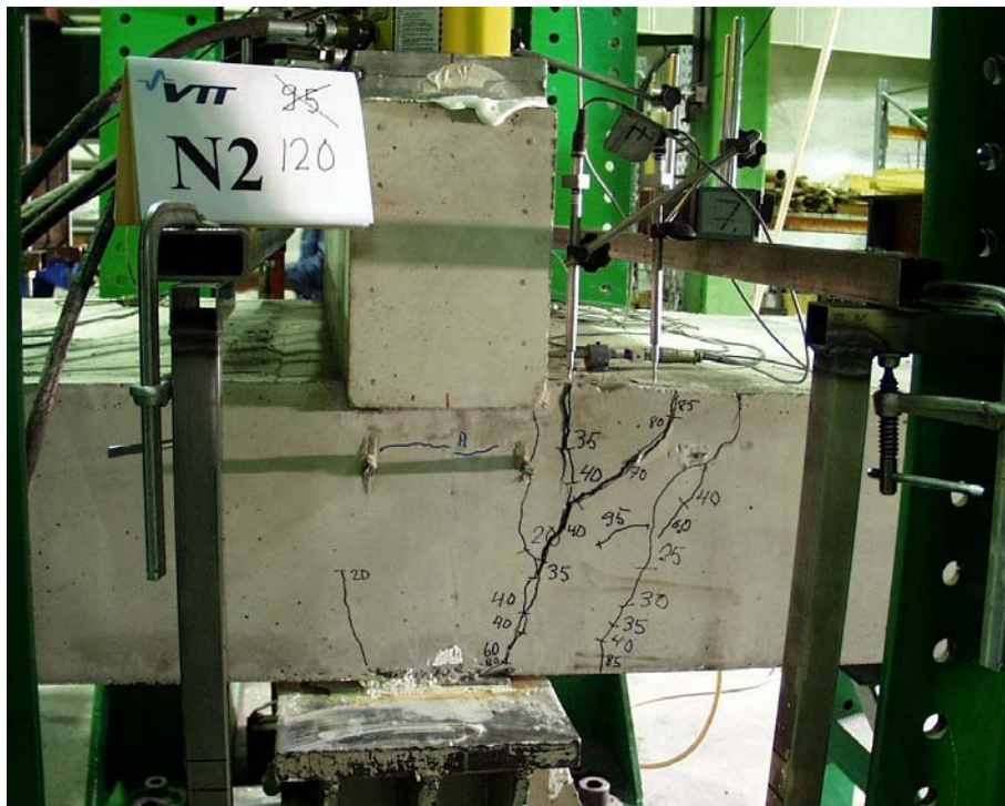
Fig. 24. N2, North edge. Cracks before failure.
