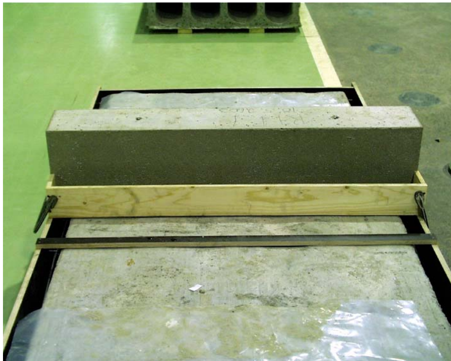
Fig. 4. N1. Preparations for grouting of upper part of joint.
