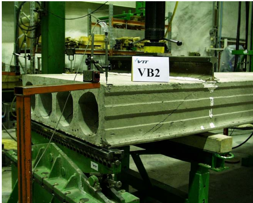
Fig. 1. VB2, North edge after failure.
