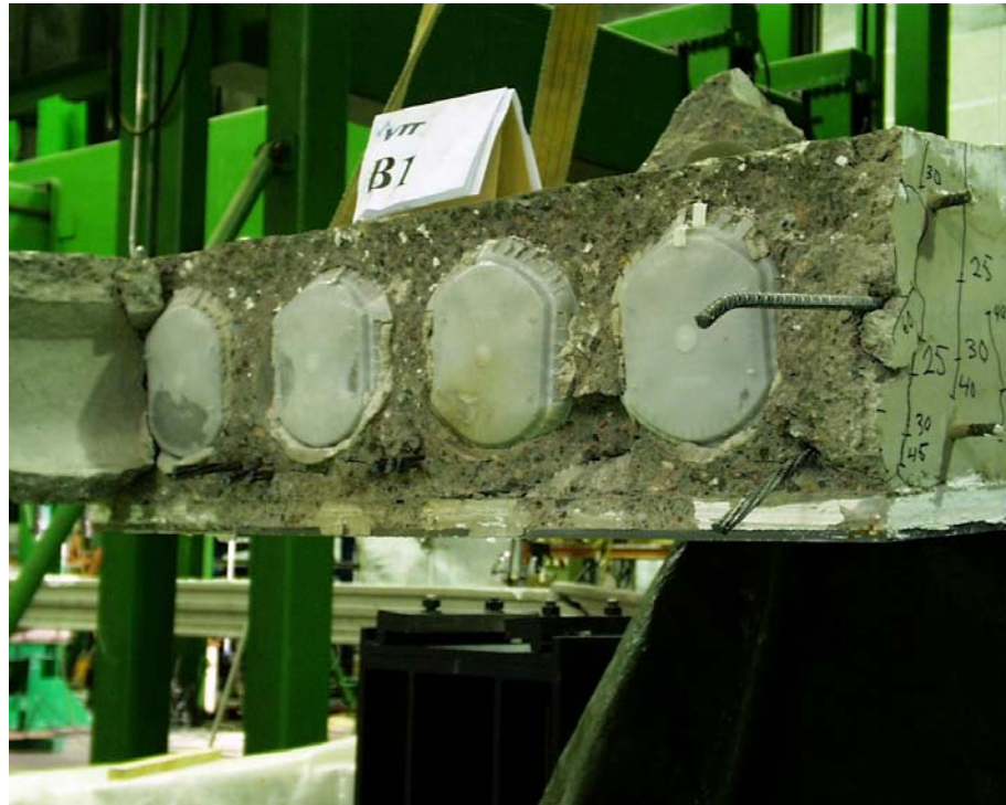
Fig. 21. B1.III. Flexural crack after flame cutting the strands and tie bars.
