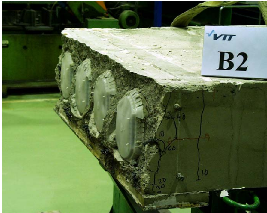
Fig. 35. B2. Flexural crack after flame cutting the strands and the tie bars.
