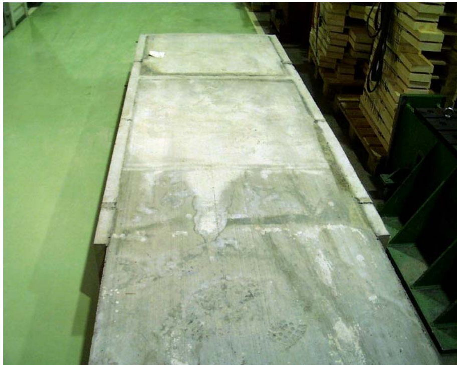
Fig. 4. Top surface after grouting.
