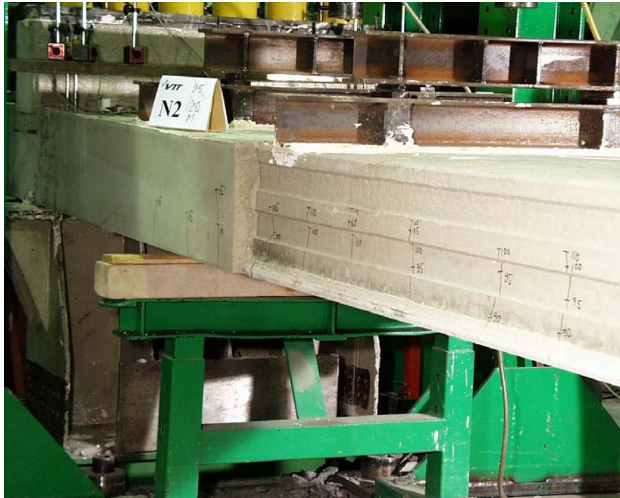
Fig. 27. N2, North edge. Failure crack and flexural cracks.
