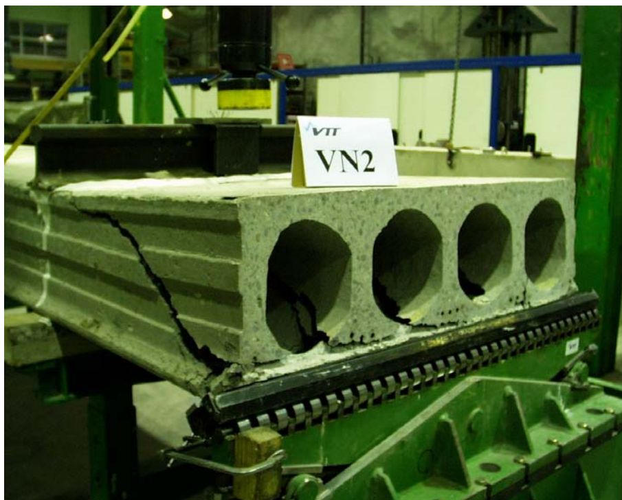
Fig. 4. VN2. South edge after failure.
