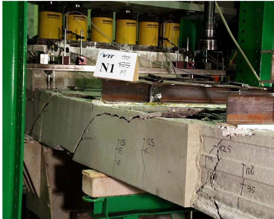
Fig. 13. N1. North edge after failure.
