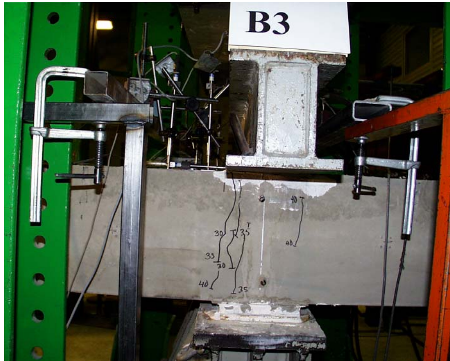
Fig. 37. B3, South edge. First cracks.
