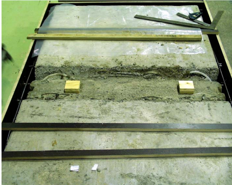
Fig. 3. N1. Joint after grouting of lower part of joint.
