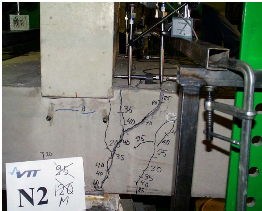
Fig. 28. N2, North edge. Cracks next to the joint after failure.
