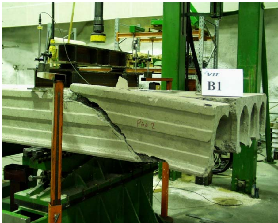
Fig. 14. B1.III, North edge. Arrangements at simply supported end after failure in test B1.II.
