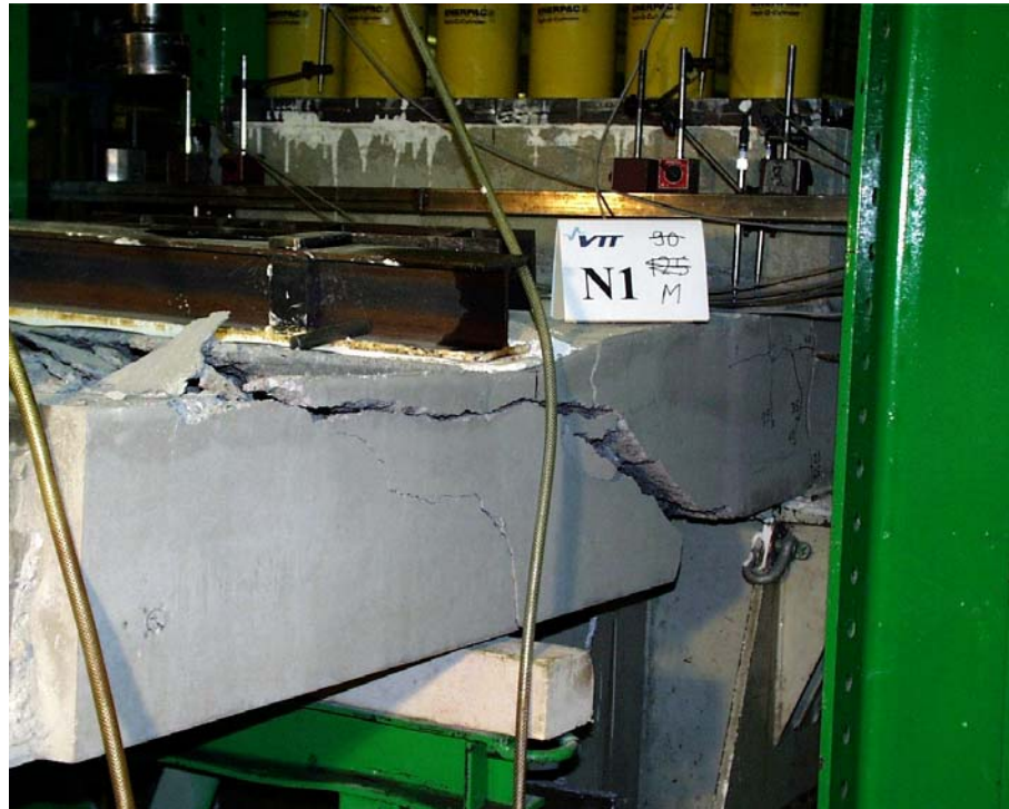
Fig. 15. N1. South edge after failure.
