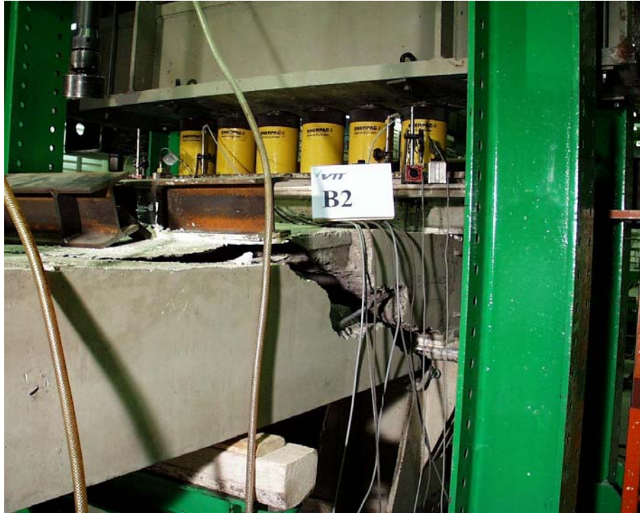
Fig. 31. B2. South edge after failure.
