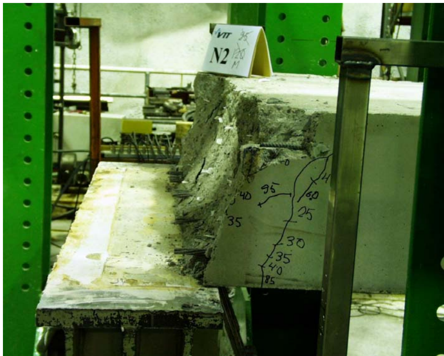
Fig. 34. N2. Flexural crack.
