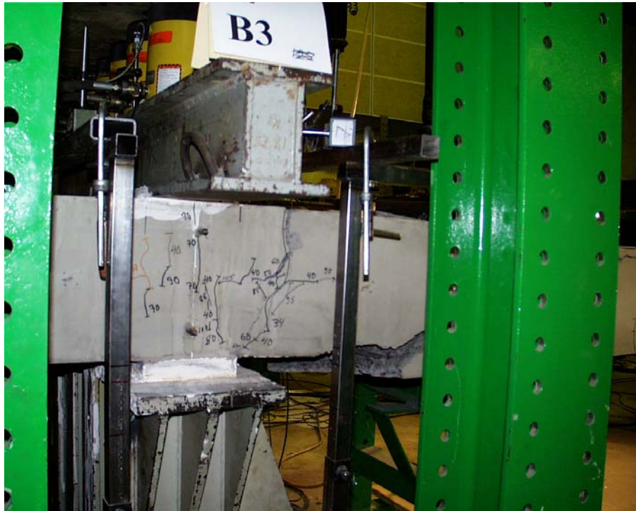
Fig. 41. B3. North edge after failure.
