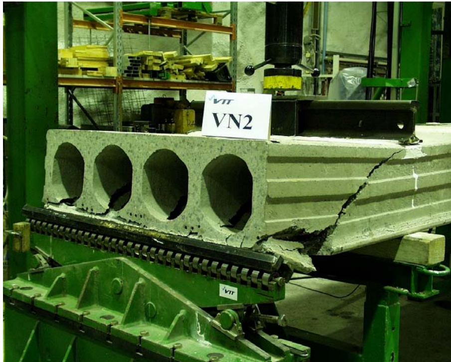
Fig. 3. VN2. North edge after failure.
