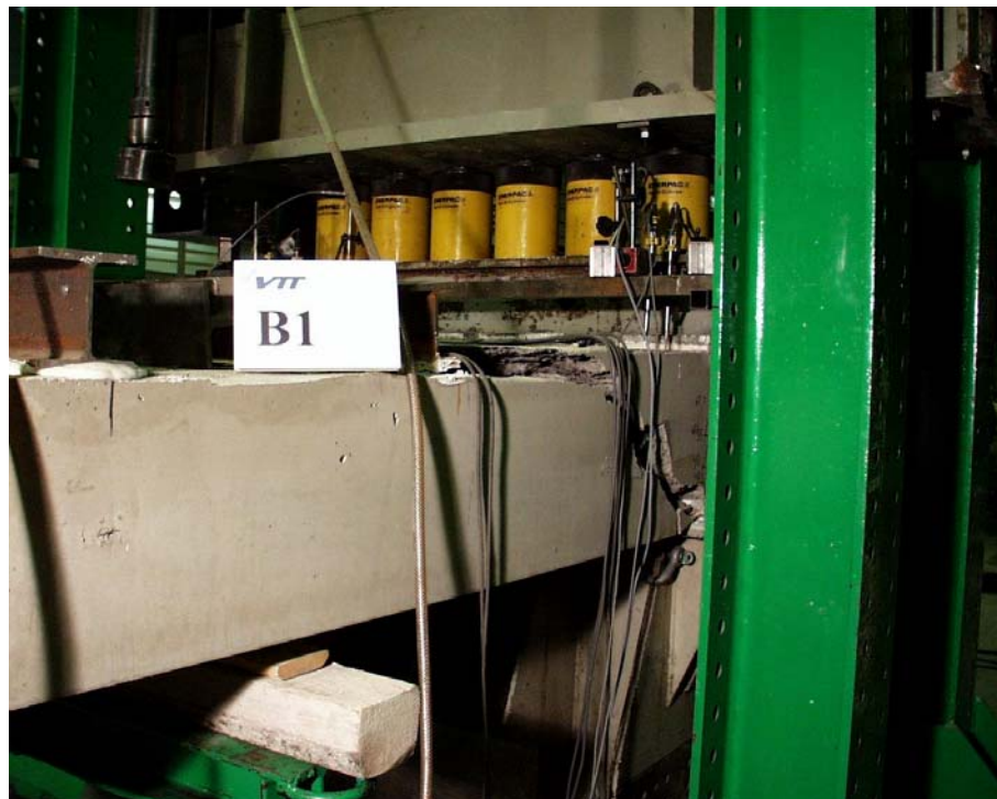
Fig. 18. B1.III. South edge after failure.
