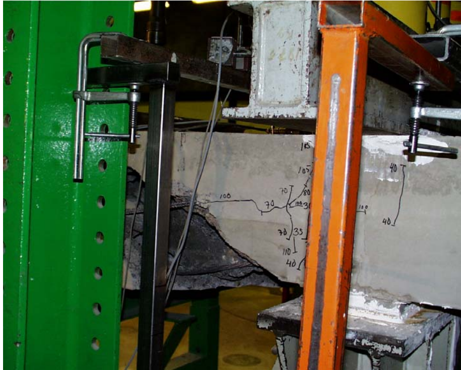
Fig. 43. B3. South edge after failure.
