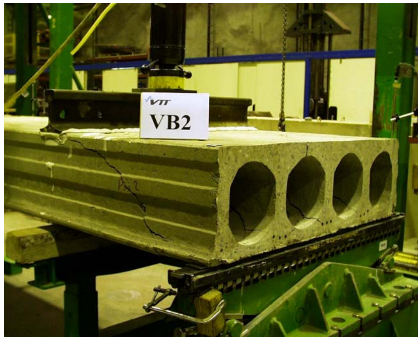
Fig. 2. VB2, South edge after failure.
