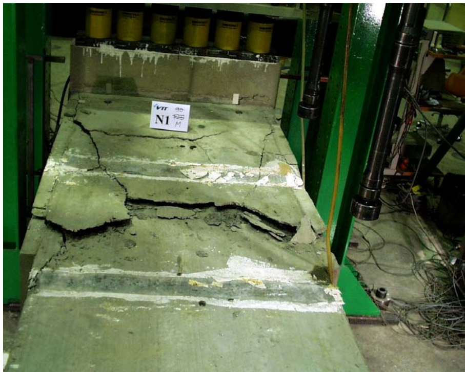
Fig. 18. N1. Top surface after failure.
