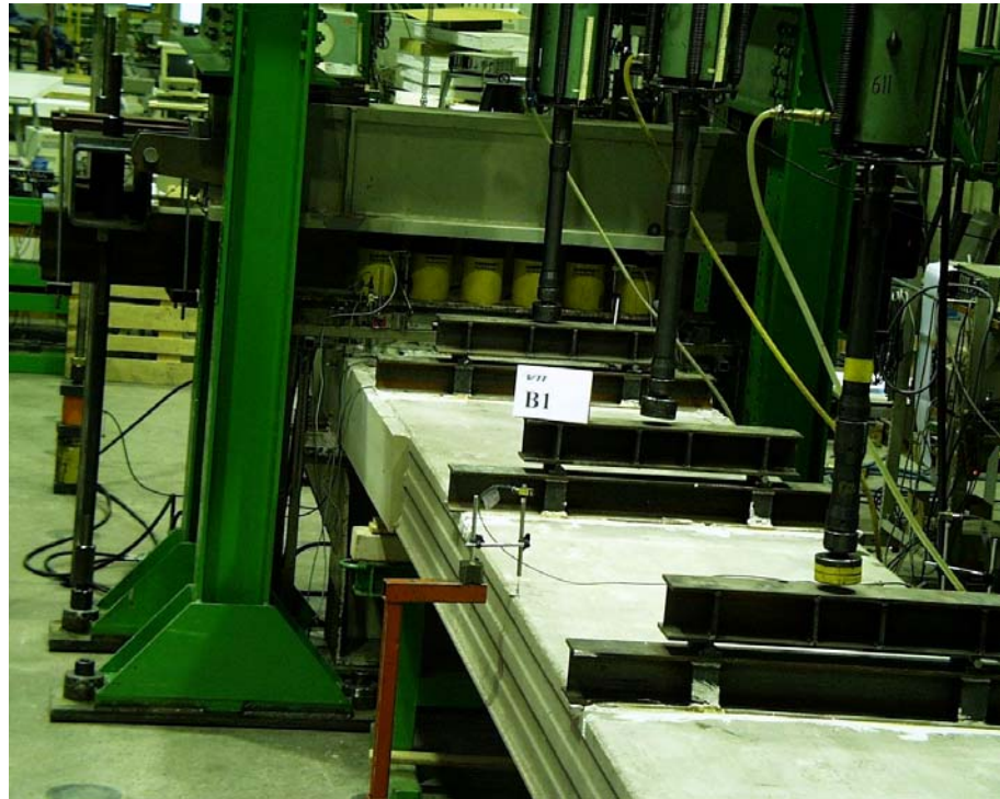
Fig. 7. B1.I. Overview on loads above the joint and next to it.
