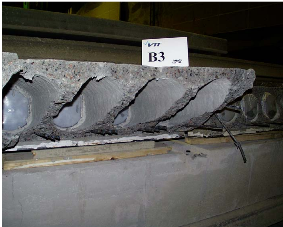
Fig. 46. B3. Shear crack after flame cutting the strands and tie bars.
