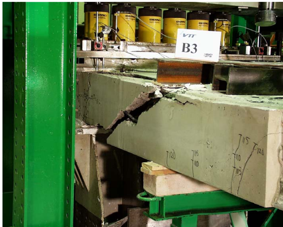
Fig. 40. B3. North edge after failure.
