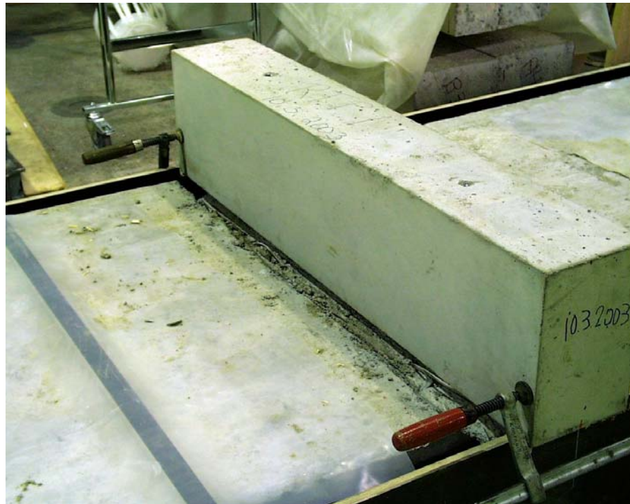
Fig. 5. NI. Grout coming from the opposite side of the wall element.
