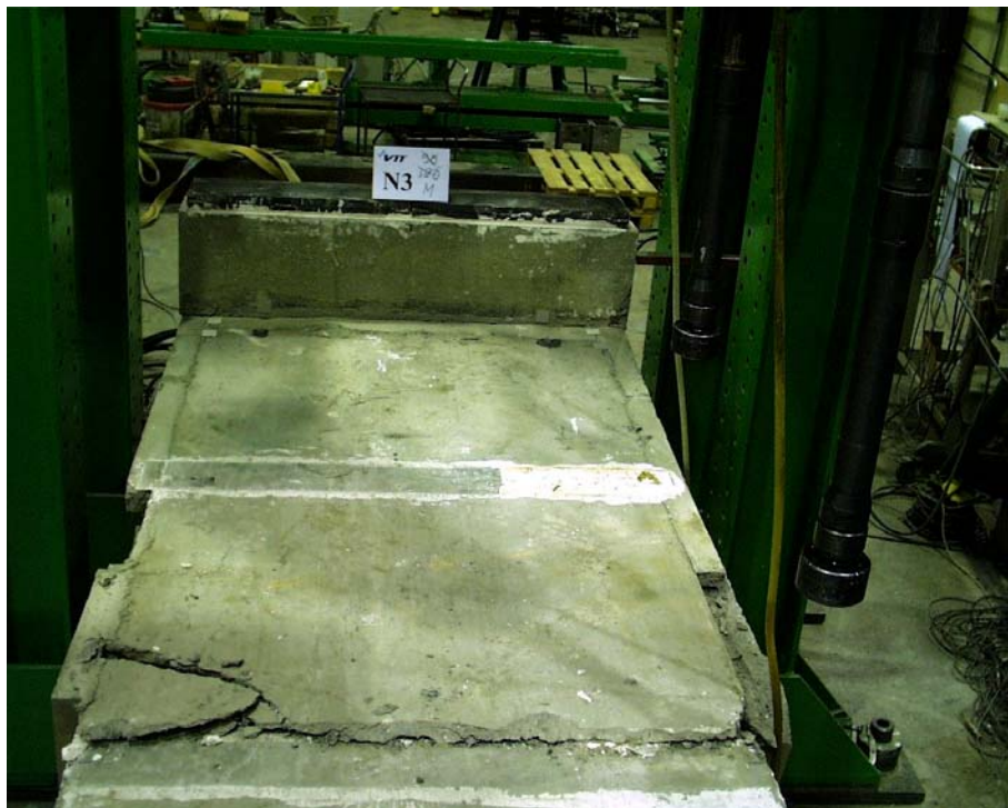
Fig. 44. N3. Top surface after failure.
