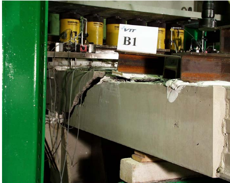
Fig. 15. B1.III. North edge after failure.
