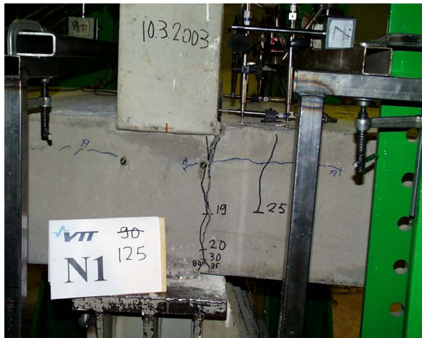
Fig. 10. N1, North edge. Cracks before failure.
