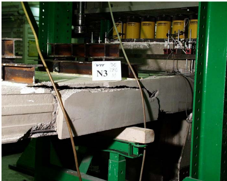
Fig. 42. N3, South edge. Failure crack and flexural cracks.
