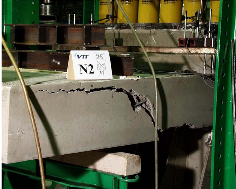
Fig. 29. N2, South edge. Failure crack.
