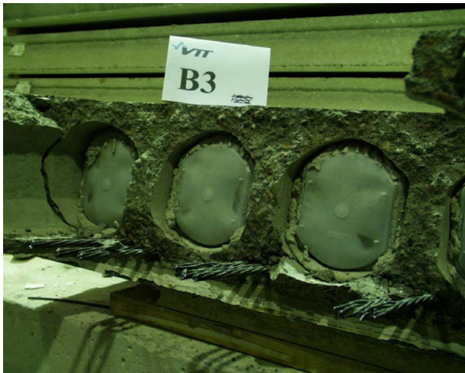
Fig. 48. B3. Detail of flexural crack.
