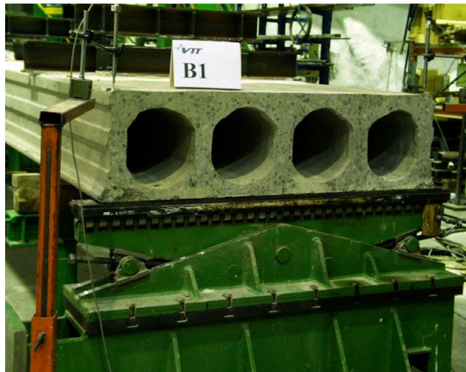
Fig. 8. B1.I. Arrangements at non-jointed end of slab.
