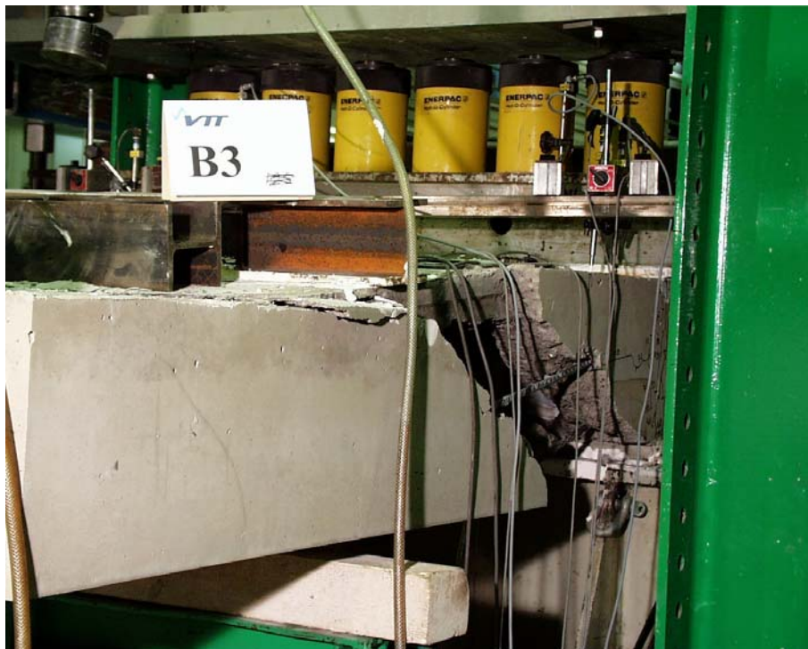
Fig. 42. B3. South edge after failure.
