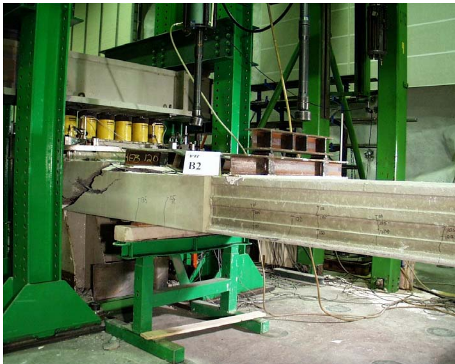
Fig. 32. B2. Flexural cracks.
