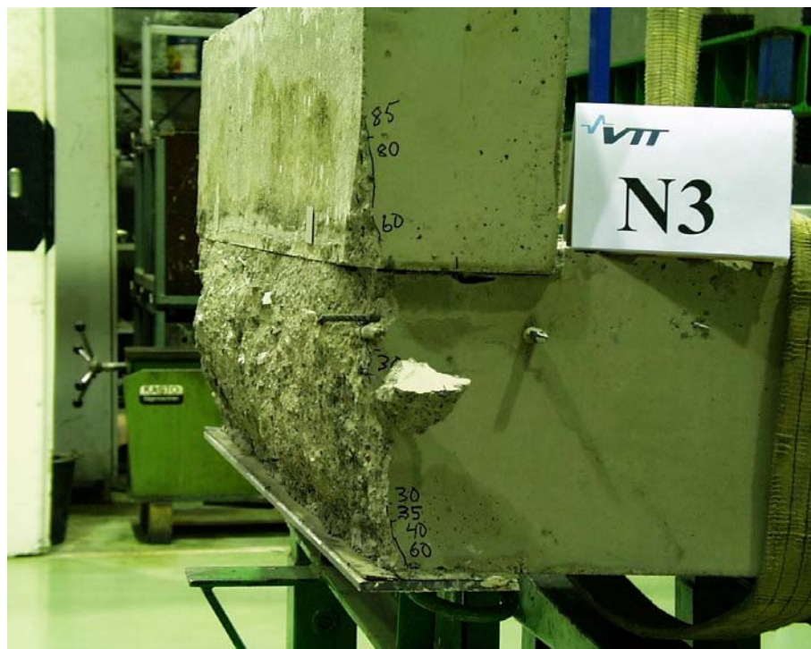
Fig. 46. N3. Flexural crack.
