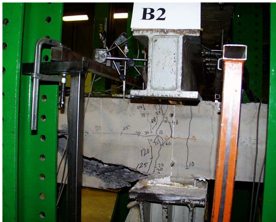
Fig. 29. B2. North edge after failure.
