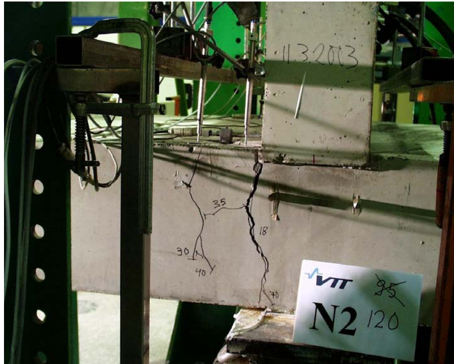
Fig. 25. N2, South edge. Cracks before failure.
