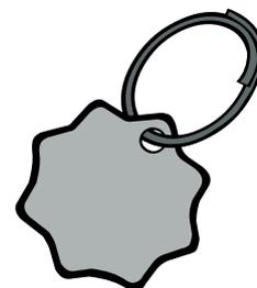
*The markings on chain slings (maximum load and allowed lifting angles, CE marking, and often the periodic inspection) are typically found on the tag on the main link. If the tag/markings are missing or unreadable, you may not use the sling.*
